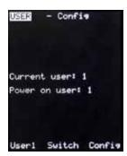
The User main mode is for configuration. It does not display any information about the signals plugged into the O'Tool. It is used to change users and to set configuration settings.
